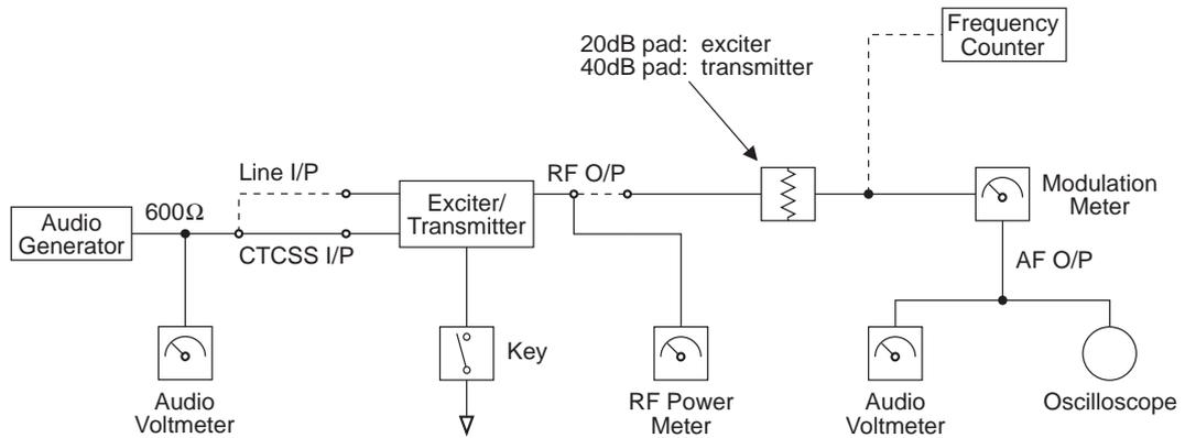
Figure 3.2 T826/827 Test Equipment Set-up
